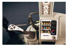
**Pilot Actuated Loader Joystick**
