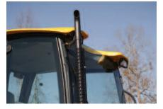
Corner Exhaust/Front Roof Cut-out
